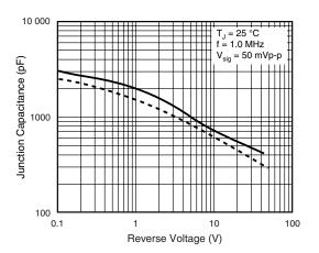
Figure 5. Typical Junction Capacitance Per Diode
