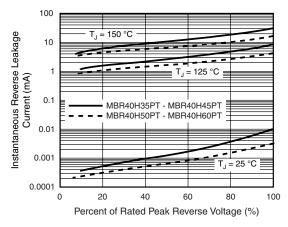
Figure 4. Typical Reverse Characteristics Per Diode
