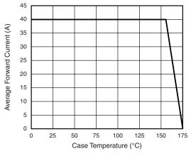
Figure 1. Forward Current Derating Curve
